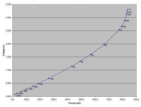
Figure 2. Voltage versus Current for Various External Pull-up Resistors on PB0
