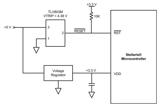
Figure 6. Using a Voltage Supervisor to Monitor the Voltage Rail
