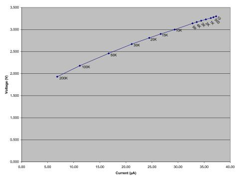
Figure 3. Voltage versus Current for Various External Pull-up Resistors on PB1
