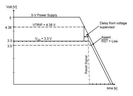
Figure 7. Resulting Waveform Using the Voltage Supervisor Circuit
