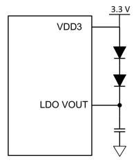
Figure 8. Diode Stack between VDD and LDO
