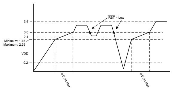
Figure 5. VDD Waveform Signature Limits
