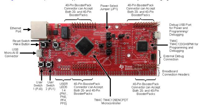
Figure 1-1. TM4C Series Crypto Connected LaunchPad Evaluation Board
