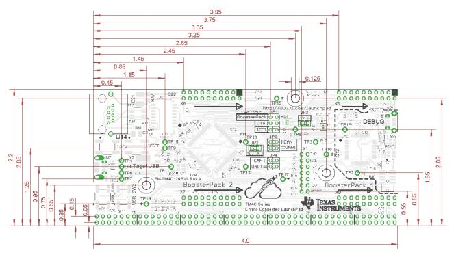
Figure A-1. Crypto Connected LaunchPad Dimensions and Component Locations
