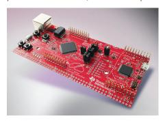
applications. The design highlights the TM4C1294NCPDTI MCU with 120-MHz 32-bit ARM Cortex-M4 MCU with Ethernet MAC+PHY, 1MB Flash, 256KB SRAM and more.
