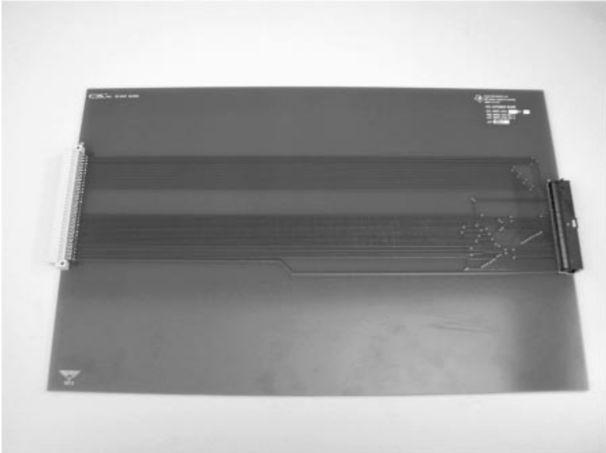
Figure 4. RIP 2.0 Extender Board
