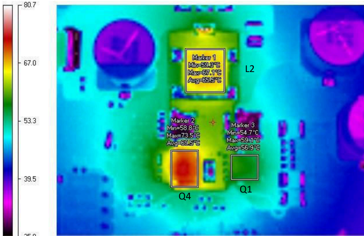
Figure 4-3. Thermal Performance: V_{IN} = 2.5\text{ V} , V_{OUT} = 8.5\text{ V} , I_{OUT} = 4\text{ A} , No Forced Airflow
