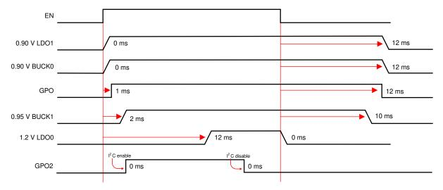
Figure 1. LP873347 Power-up and Power Down Sequence
