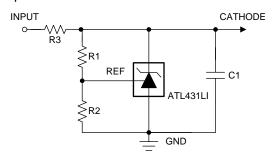
Figure 3. Base Shunt Regulator Schematic
