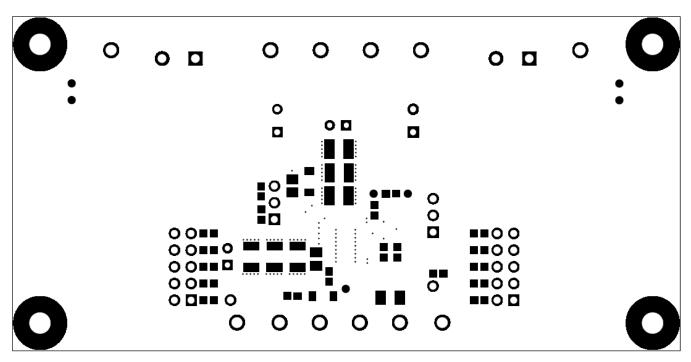
Figure 16. LMZ34202EVM Bottom Solder Mask
