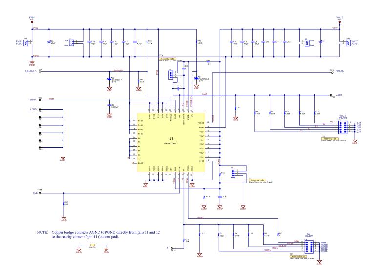
Figure 8. LMZ34202EVM Schematic
