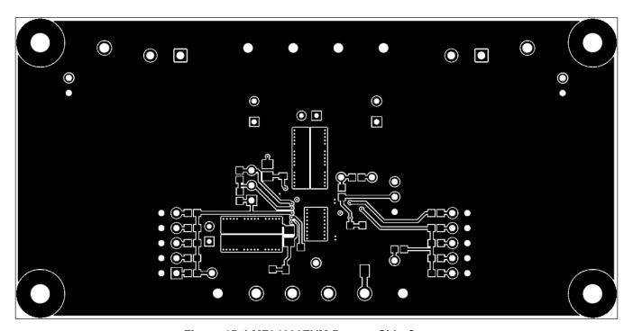
Figure 15. LMZ34202EVM Bottom-Side Copper
