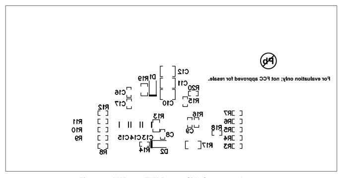
Figure 17. LMZ34202EVM Bottom-Side Component Layout
