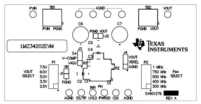
Figure 10. LMZ34202EVM Topside Component Layout
