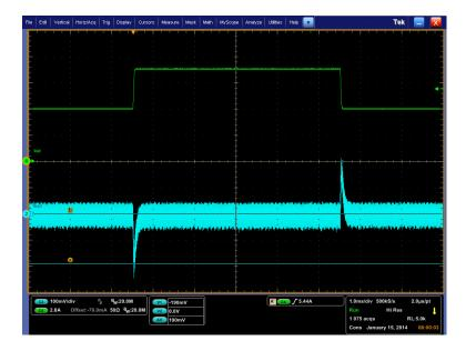
57Vin @ 4A to 7A, 100mA/ $\mu$ s, Pulse f @ 100 Hz, 50% duty cycle, 12V out. Load Step on/off.
