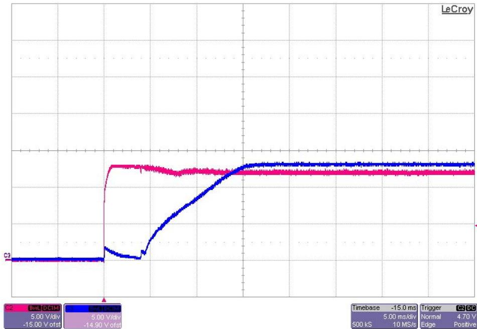
The photo below shows the output voltage startup waveform after the application of 6V in. The 13.2V output was loaded to 0A. (5V/DIV, 5mS/DIV)
