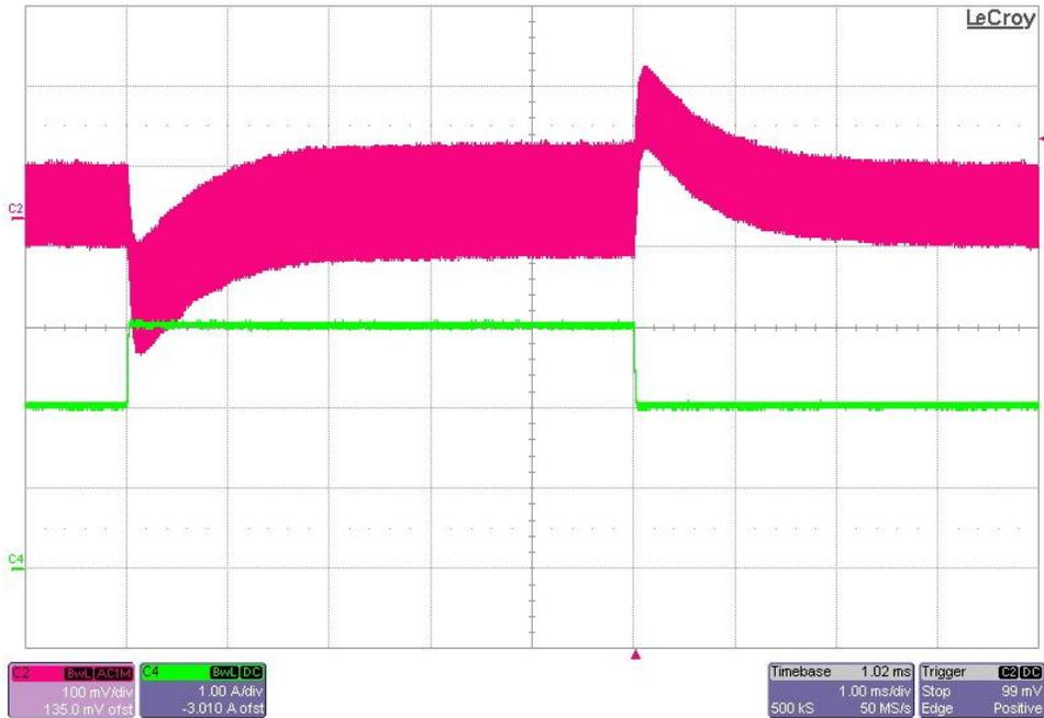
The photo below shows the 13.2V output voltage (ac coupled) when the load current is stepped between 0.5A and 3A.  $V_{in} = 12V$ . (200mV/DIV, 1A/DIV, 1mS/DIV)
