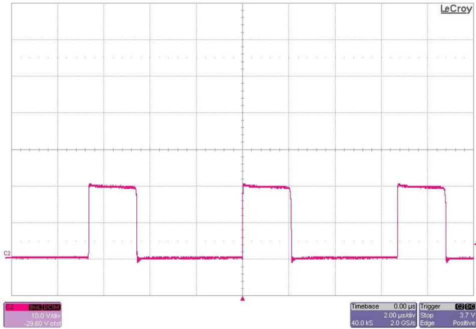
The photo below shows the FET switching voltage (TP4) for an input voltage of 16V and a 1.1A load. The converter is operating in DCM. (10V/DIV, 2uS/DIV)
