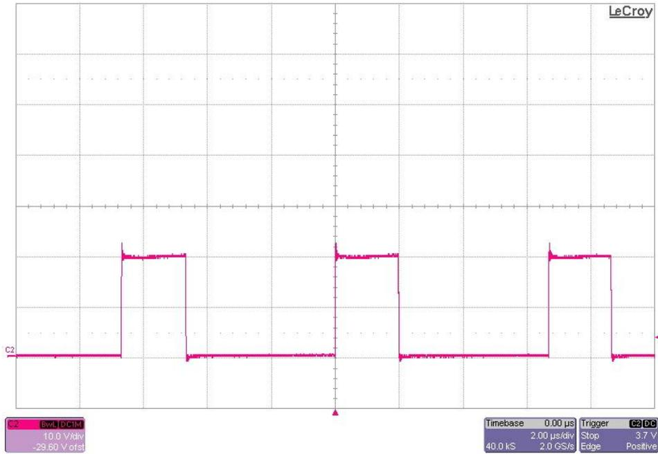
The photo below shows the FET switching voltage (TP4) for an input voltage of 16V and a 3A load. (10V/DIV, 2uS/DIV)
