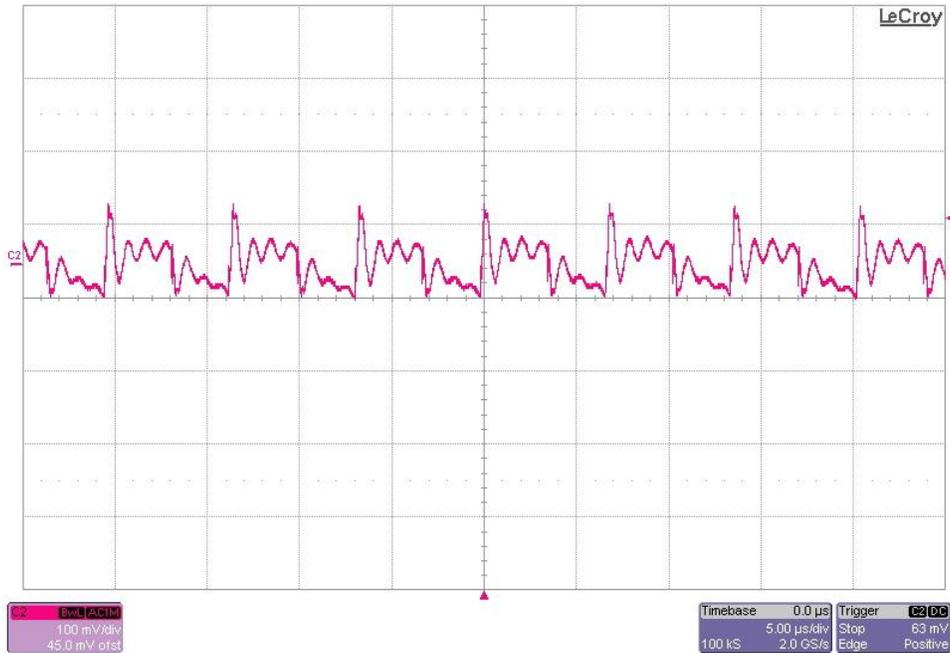
The 13.2V output ripple voltage (AC coupled) is shown in the figure below. The image was taken with the output loaded to 3A. The input voltage is set to 12V. (100mV/DIV, 5uS/DIV)
