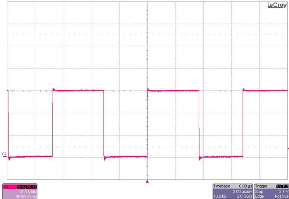
The photo below shows the FET switching voltage (TP4) for an input voltage of 6V and a 0.35A load. The converter is operating in DCM. (10V/DIV, 2uS/DIV)
