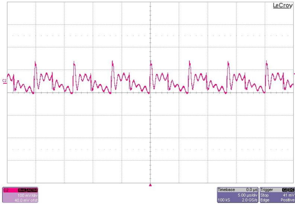
The 13.2V output ripple voltage (AC coupled) is shown in the figure below. The image was taken with the output loaded to 1A. The input voltage is set to 12V. (100mV/DIV, 5uS/DIV)
