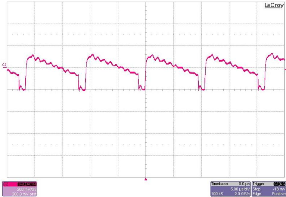
The 120V output ripple voltage is shown in the figure below. The image was taken with the output loaded to 10mA and the input voltage set to 36Vdc. (200mV/DIV, 5uS/DIV)
