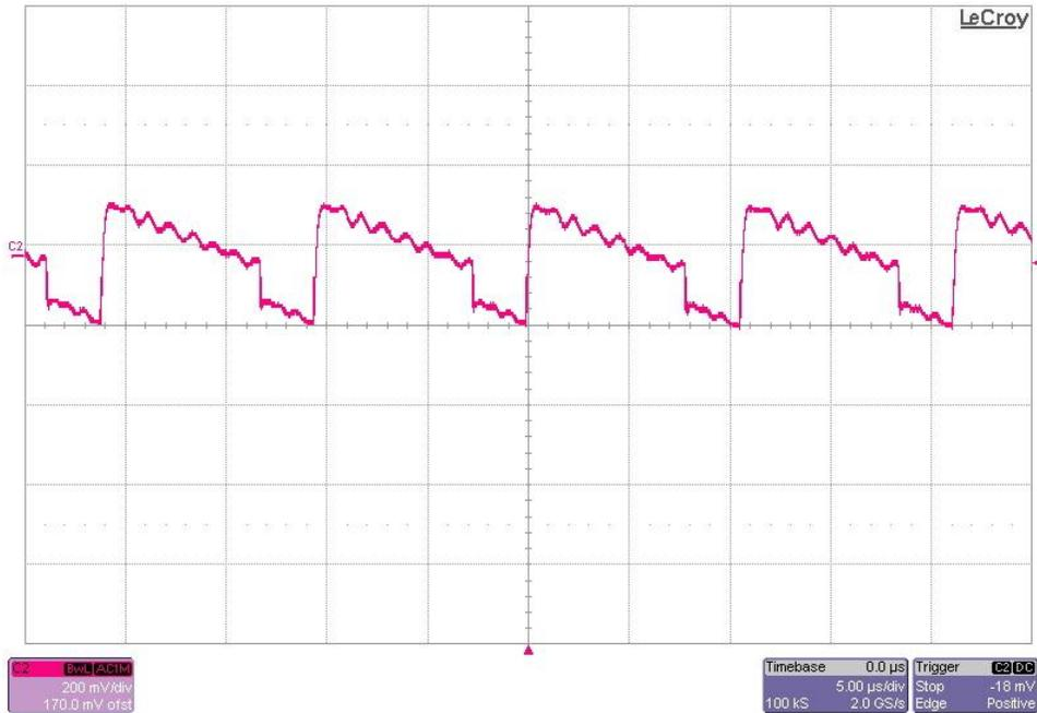
The 120V output ripple voltage is shown in the figure below. The image was taken with the output loaded to 10mA and the input voltage set to 24Vdc. (200mV/DIV, 5uS/DIV)
