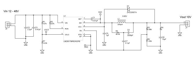
Figure 1. Complete Evaluation Board Schematic for LM25017 Based Synchronous Buck Converter
