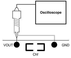
Figure 3. Voltage Ripple Measurements
