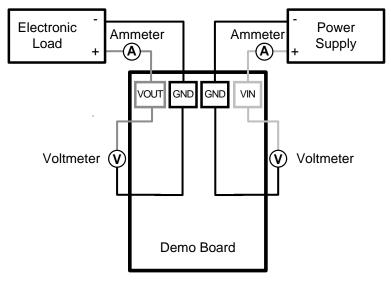
Figure 2. Efficiency Measurements
