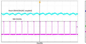
Figure 4. TPS564242 12-V Input to 5-V Output at 4 A
