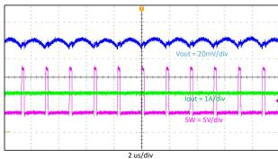
Figure 5. TPS563202 12-V Input to 5-V Output at 3 A
