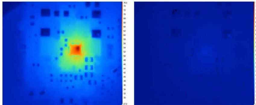
**Figure 3. Heat Generation at the High-Side Switch During Operation**
