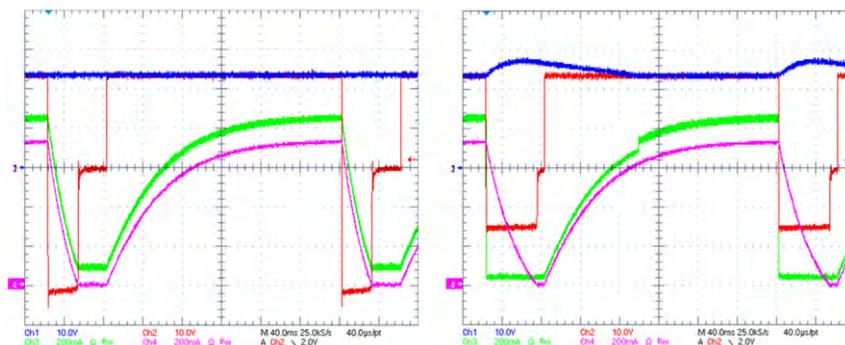
**Figure 2. Voltage and Current Curves of Standard and Improved Inductive Discharging**
