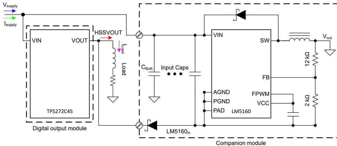
**Figure 1. Improved Inductive Discharge Concept Block Diagram**
