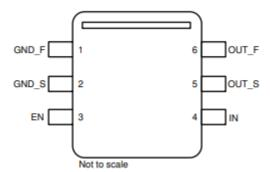
Figure 4-1. Pin Diagram (DBV-6) Package
