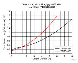
Figure 2. TPS54824 Reduced Power Loss Over TPS54620
