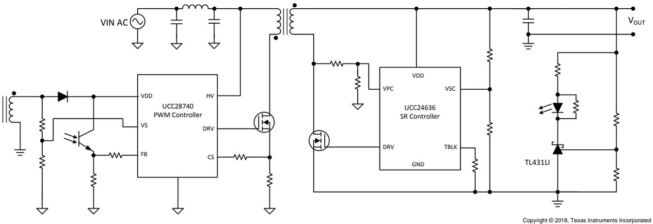
Figure 1. Schematic Diagram for a Flyback Converter
