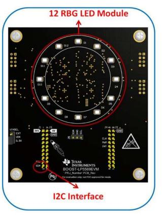
Figure 1. LED Board Design
