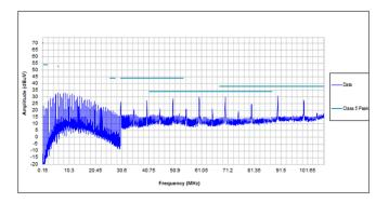
Figure 63. Conducted Emissions for 400-kHz Return
