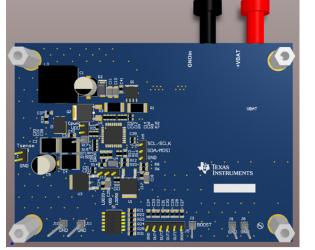
Figure 2. Top View of LP8860-Q1 EMI Test Board
