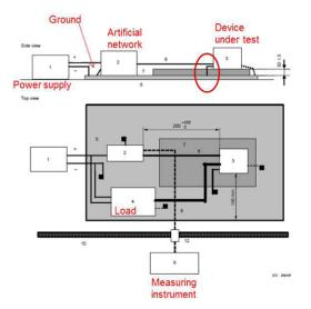
Figure 4. Schematic of LP8860-Q1 EMI Test Board
