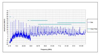
Figure 62. Conducted Emissions for 400-kHz Line
