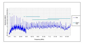
Figure 60. Conducted Emissions for 2.2-MHz Line
