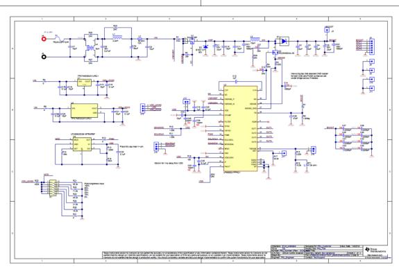
Figure 3. Schematic of LP8860-Q1 EMI Test Board
