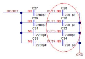
Figure 39. Circuit With Capacitors Between LED Drivers and GND
