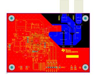
Figure 1. Top Layer of PCB Layout of LP8860-Q1 EMI Test Board
