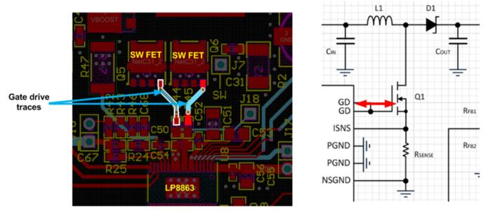
Figure 12. Gate-Drive Signal From LP8863-Q1 to SW FET
