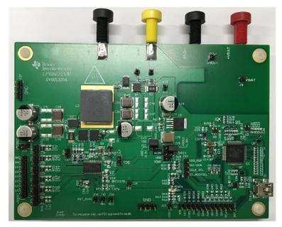
Figure 3. Top View of LP88663-Q1 EVM
