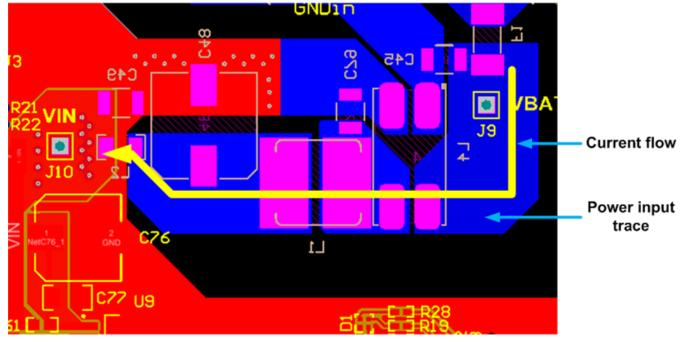
Figure 18. Boost Input Power (V<sub>IN</sub>) Trace
