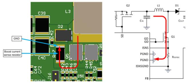
Figure 5. Switching Current Loop 1
