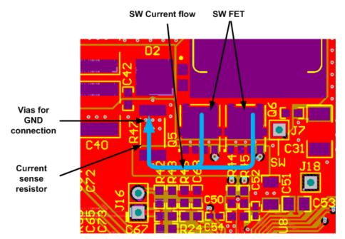
Figure 9. Vias for Ground Plane Connection
