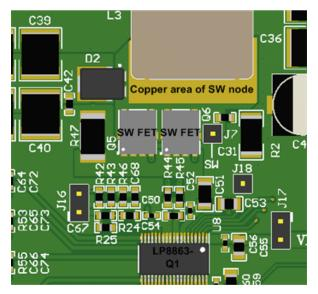
Figure 8. Copper Area of SW Node for Thermal Dissipation
