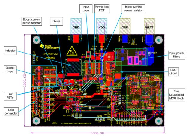
Figure 2. PCB Layout of LP8863-Q1 EVM
