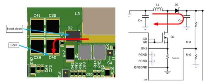
Figure 6. Switching Current Loop 2
