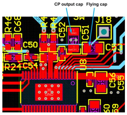
Figure 16. Capacitor Locations of Charge Pump
