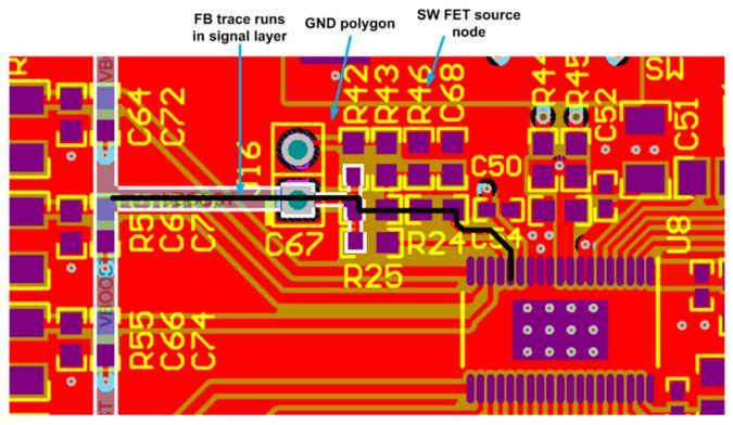
Figure 15. Trace for Boost Feedback
