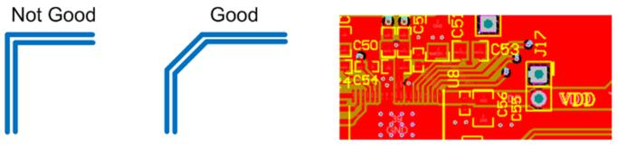
Figure 20. Recommended Trace Routing of Digital Signals
