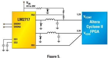
LM2717 1.2V Core, 3.3V I/O Dual Integrated Switching FPGA Supply Using an LM4040 Shunt Reference for Sub-1.25V Core Voltage Generation
