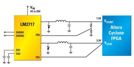
Figure 1. LM2717 Dual Integrated Switching Supply for 1.5V Core and 3.3V I/O Medium-power FPGA
