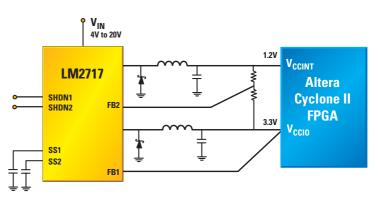
Figure 4. LM2717 1.2V Core, 3.3V I/O Dual Integrated Switching FPGA Supply Using the 3.3V Rail as Auxiliary Voltage for Sub-1.25V Core Voltage Generation
