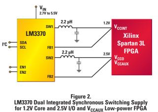
*Figure 2* shows a low-power 1.2V, 90 nm FPGA (Spartan 3L from Xilinx) powered by the LM3370, a dual 600 mA per channel integrated synchronous buck regulator.
