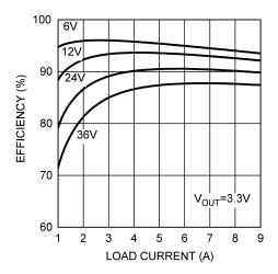
Figure 7. Typical Efficiency vs Load Current
