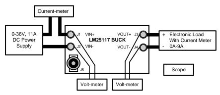
Figure 1. Typical Evaluation Setup
