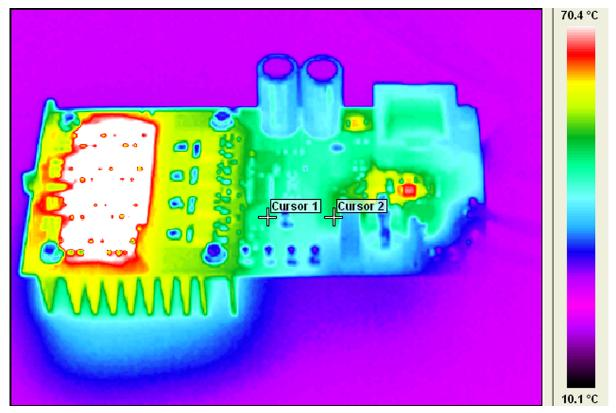
Figure 13. Top Side Thermal Scan
