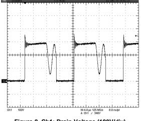
Figure 8. Ch1: Drain Voltage (100V/div) Time (4 µs/div)
