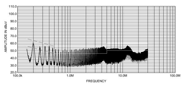
Figure 12. Peak Conductive EMI scan per CISPR-22, Class B Limits
