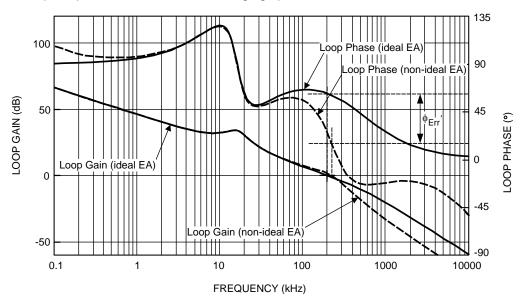
Figure 6. Overall Loop T<sub>v</sub>(s) Bode Plot With Ideal and Actual EA
