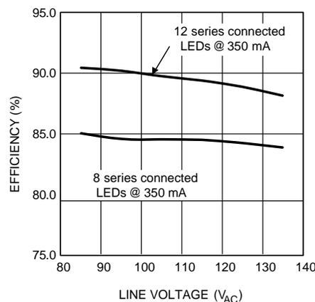
**Figure 4. LM3445 Efficiency vs Input Voltage
