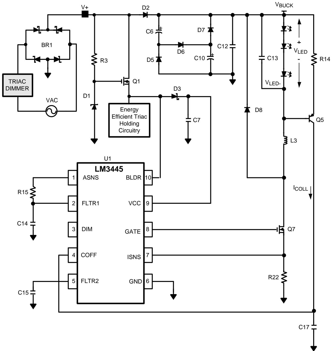
Figure 1. LM3445 Schematic
