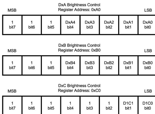
**Figure 10. Brightness Control Register Description**
