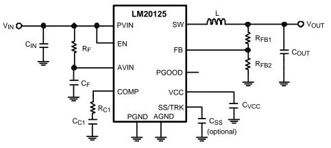
Figure 1. 3.3V Output Solution Optimized for Size and Efficiency
