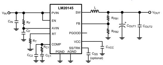
Figure 5. 1.2V Output Solution Optimized for Load Transients
