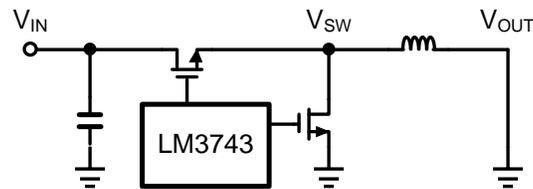
**Figure 3. Output Short-Circuit to Ground**
