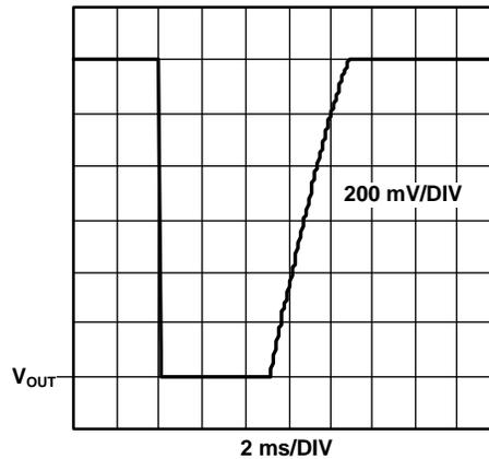
**Figure 2. Hiccup Time Out and Internal Soft-Start**
