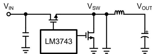
**Figure 4. Switch Node Short-Circuit to Ground**
