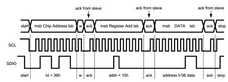
NOTE: w = write (SDIO = "0"): r = read (SDIO = "1"): ack = acknowledge (SDIO pulled down by either master or slave): id = chip address, 36h for LM27965
