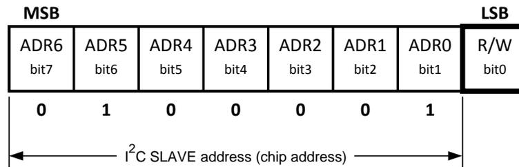
**Figure 5. Device Address**
