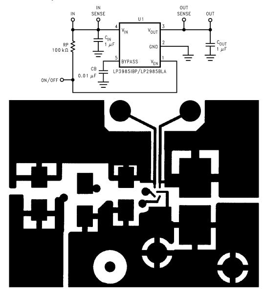
**Note**: The board layout for the large bump and the small bump DSBGA-5 is the same. Only the footprints are different.
