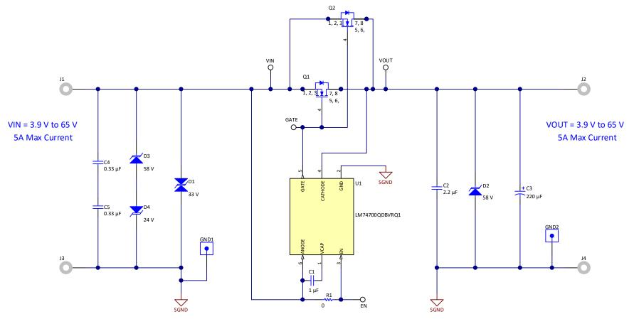
Figure 3. LM74700EVM Schematic
