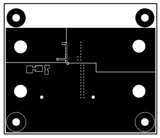
Figure 11. LM74700EVM Bottom Layer Routing
