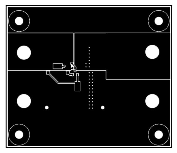
Figure 10. LM74700EVM Top Layer Routing
