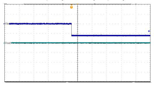
Figure 5. Startup Reverse Polarity (-12 V)
