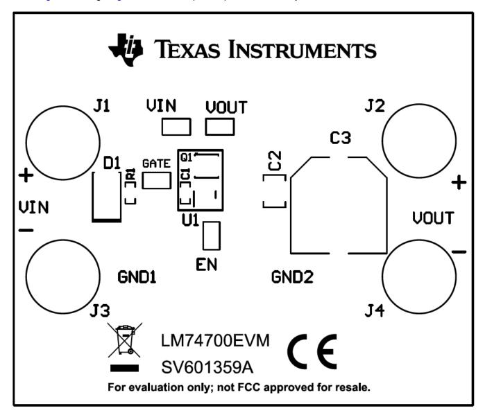
Figure 8. LM74700EVM Top Side Placement
