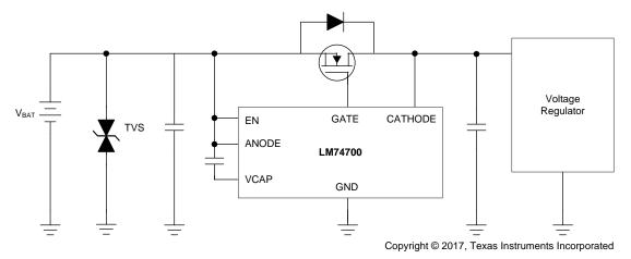
Figure 1. LM74700EVM Typical Application Circuit
