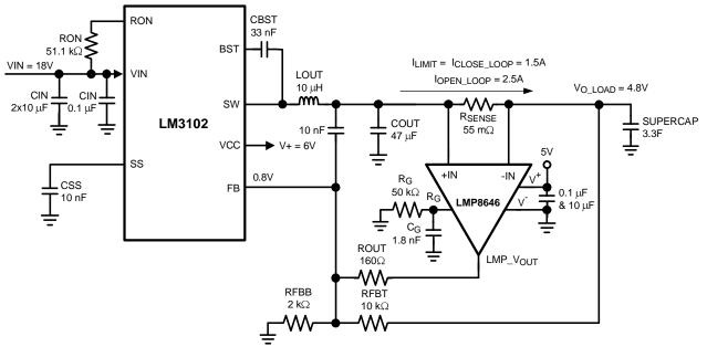
Figure 2 – Schematic for the SuperCap Application
