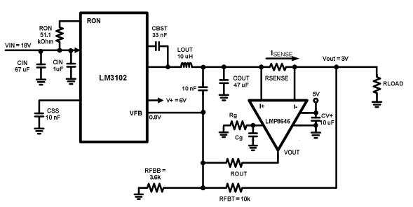
Figure 5 – Recommended Components for the LM3102
