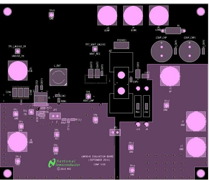
Figure 10 - Layout Layer #2: Power
