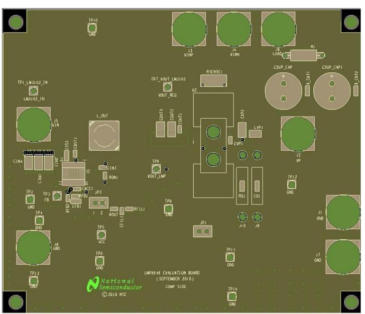
Figure 11 - Layout Layer #3: Ground
