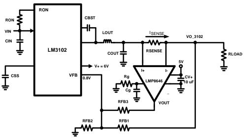
Figure 4 – Schematic for the Resistive Load Application
