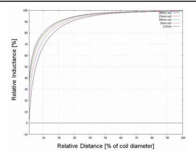
Figure 2-2. Relative Inductance vs Distance of Various Coil Sizes
