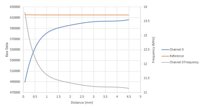
Figure 4-3. Measured Raw Data of LDC3114 With Sensor R
