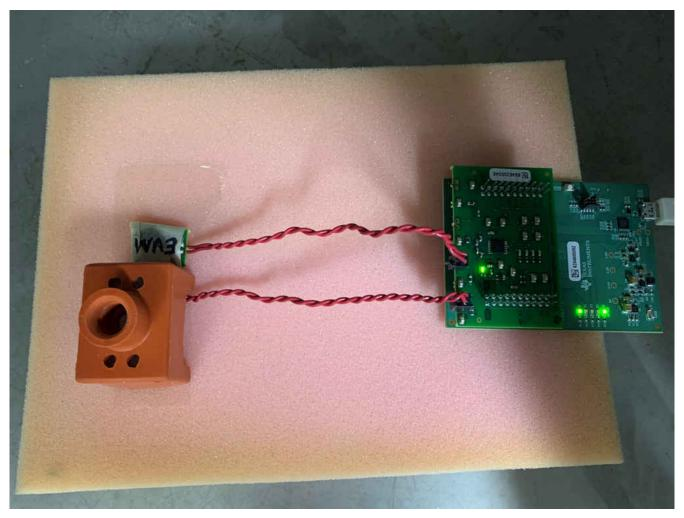
Figure 5-1. LDC3114EVM Temperature Chamber Setup
