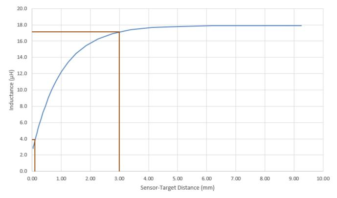
Figure 3-2. Calculated Inductive Response of LDC3114 With LDC3114EVM Coil
