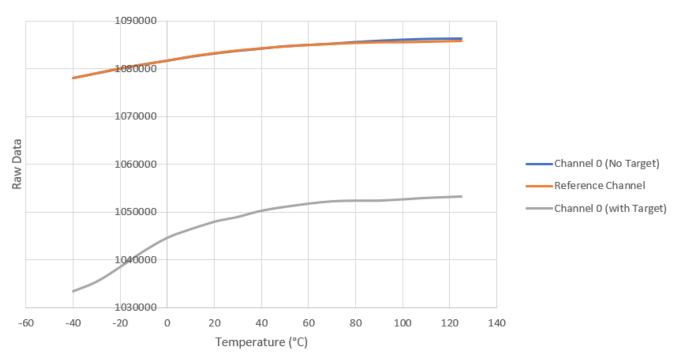
Figure 5-2. Observed Effect of Ambient Temperature on LDC3114 With LDC3114EVM Coil
