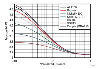
Figure 2-1. Sensor Frequency vs Distance of Common Targets
