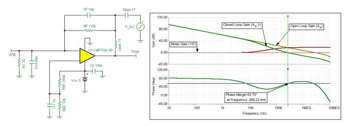
The loop gain plot shows the loop closure point (loop gain is 0 dB) at 269.22 kHz with 63.70 degrees of phase margin.
