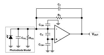
From this illustration it is apparent that  $C_{PD}$ ,  $C_{D}$ , and  $C_{CM}$  are in parallel and the capacitance at the inverting input is described by the following equation:
