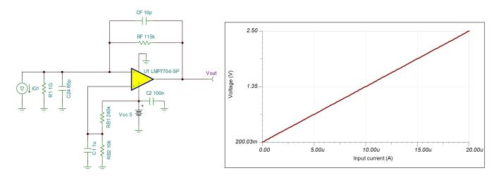
For zero input current, the simulated output voltage is 200.032 mV, and at 20- $\mu$ A input current, the simulated output voltage is 2.500 V and the gain is 115 kV/A.
