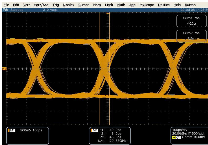
Figure 2.2 – Eye Diagram of Setup 1
