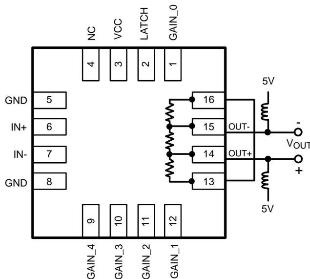
Figure 5. Alternate Connection for Low-Gain Mode (200Ω Load)
