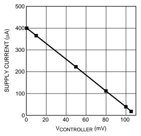
Figure 3. Power-Mode Control ( $R_{EXT} = 20\Omega$ ).
