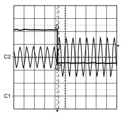
Figure 4. Output Signal With the LPV531 Op Amp
