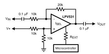
Figure 2. AC-Coupled Inverting Amplifier With the LPV531 Amplifier
