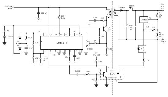
L = 15 turns #22 wire wrapped on  $\frac{1}{2}$ W resistor body. D<sub>1</sub> = optional (see text).
