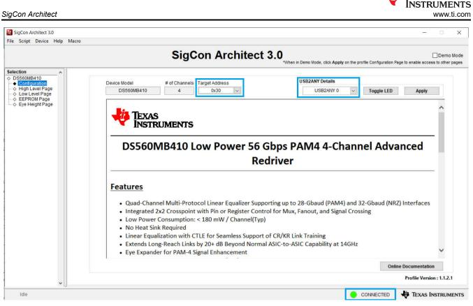
Figure 5-5. Establishing a Connection with the DS560MB410
