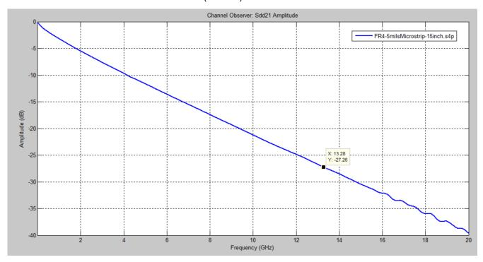
Figure 3-2. SDD21 for the 15-Inch FR4 PCB Test Trace Used at Input Channel for the Receiver Test Case
