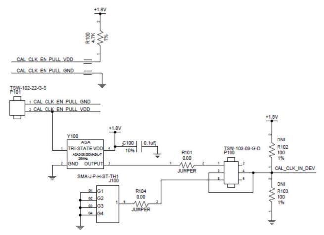
Figure 1-3. DS560DF810EVM Schematic Portion for CAL\_CLK\_IN Input Circuit; Applies to EVM Version Rev 2 and Later
