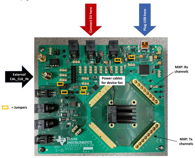
Figure 1-1. DS560DF810EVM Power, Low-Speed Communication, and High-Speed Signaling Connections
