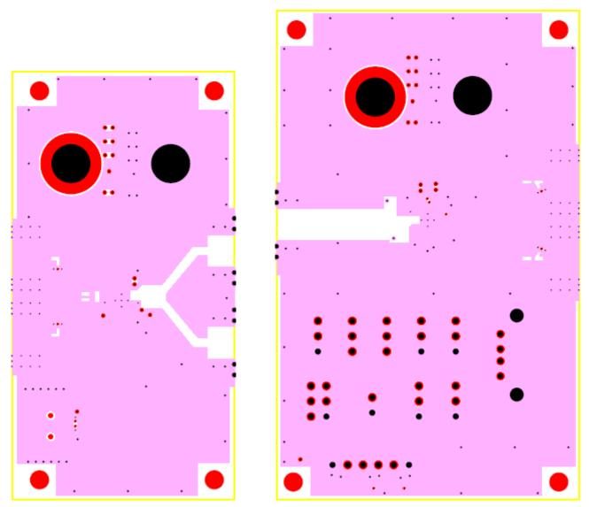
Figure 3: GND1 Layer for DRIVECABLE04-TX (left) and DRIVECABLE04-RX (right)
