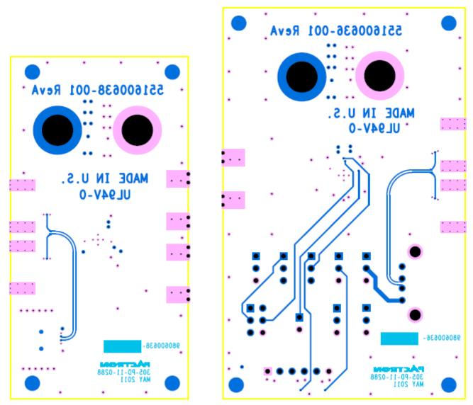
Figure 7: BOTTOM Layer for DRIVECABLE04-TX (*left*) and DRIVECABLE04-RX (*right*)
