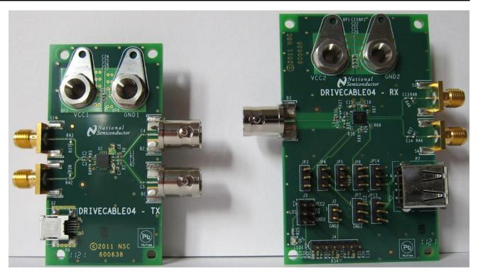
Figure 1: DRIVECABLE04-TX (left) and DRIVECABLE04-RX (right)
