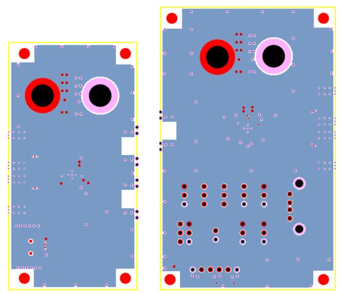
Figure 5: VCC Layer for DRIVECABLE04-TX (left) and DRIVECABLE04-RX (right)
