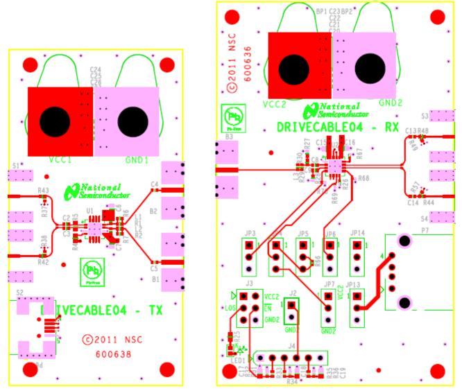
Figure 2: TOP Layer for DRIVECABLE04-TX (left) and DRIVECABLE04-RX (right)
