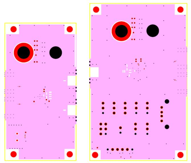
Figure 4: GND2 Layer for DRIVECABLE04-TX (left) and DRIVECABLE04-RX (right)
