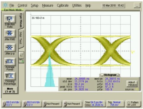
FIGURE 4. SD395 Output Waveform at 2.97 Gbps with 160m Belden 1694A Cable
