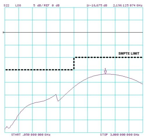
FIGURE 7. SD395 Input Return Loss
