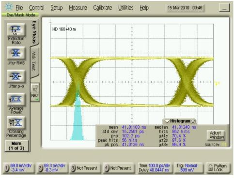
FIGURE 5. SD395 Output Waveform at 1.485 Gbps with 200m Belden 1694A Cable
