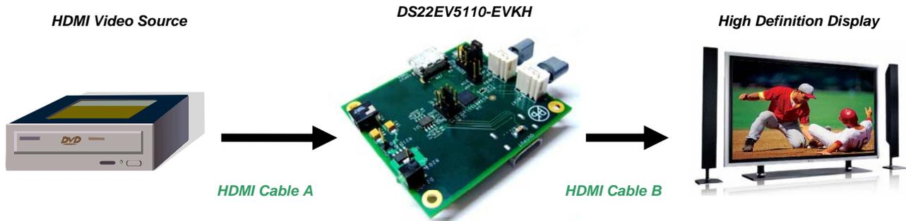
The DS22EV5110-EVKH demo kit extends TMDS with the 28 AWG STP HDMI cables as follows:
