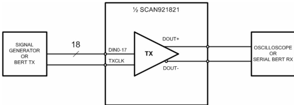
**Figure 3.** Test Setup for the SCAN921821 Only
