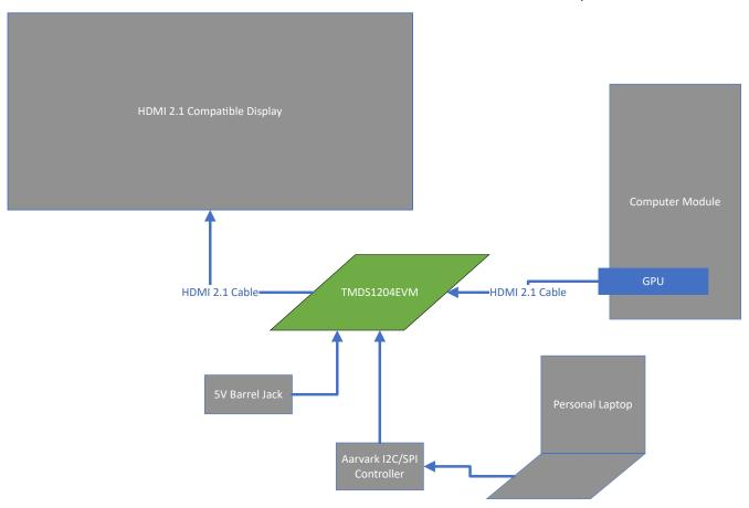
Figure 2-1. Test Setup Diagram
