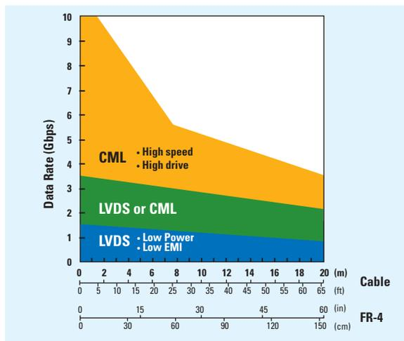
**Figure 4: Typical LVDS and CML Applications**
