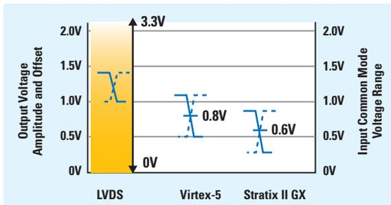
**Figure 5. Standard and FPGA Differential I/O Signaling Levels**
