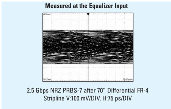
**Figure 2a. 2.5 Gbps NRZ Signal After 70 Inches of FR-4 Without Equalization**
