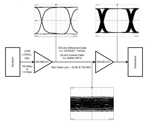
Figure 1. Typical Cable Extender Chipset Application
