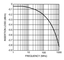
Figure 4. CAT5e Maximum Attenuation per TIA/EIA-568–B.2
