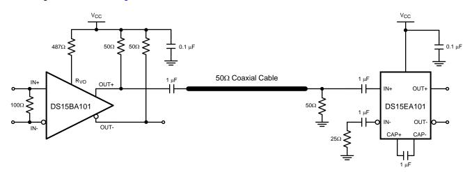
Figure 11. Cable Extender Chipset Connection Diagram for 50Ω Coaxial Cables
