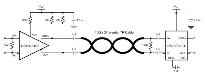
Figure 7. Cable Extender Chipset Connection Diagram for 100Ω Differential Balanced Cables
